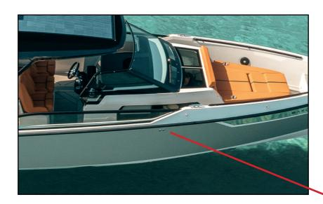
Black water tank vent and fresh water tank vent (for twin-engine option)
