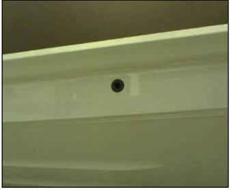
Starboard cockpit drain outlet
