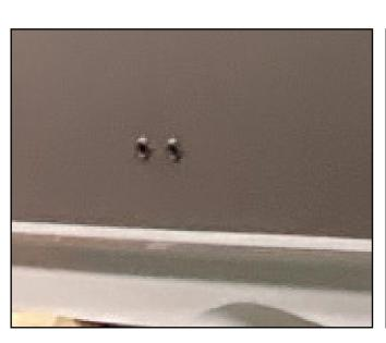
Bilge pump and air conditioner drain outlets
