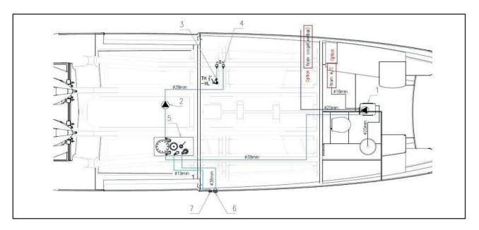
Grey water through-hull fitting indicated by number 3 and deck fitting by number 6.
