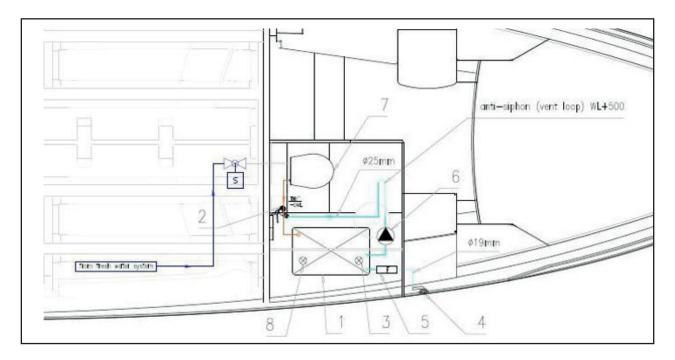
Black water through-hull fitting indicated by number 2 and deck fitting by number 3.
