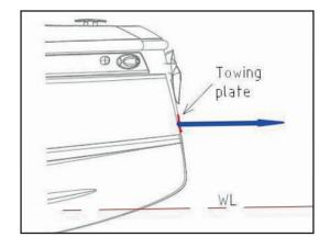
Towing using the towing plate
