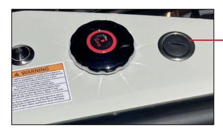
Fuel tank vent - on the right of fill point
